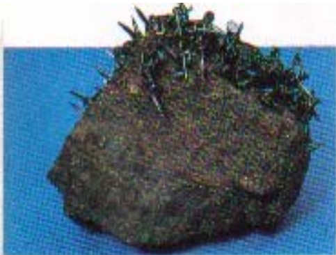
Pins, needles and nails are attracted to the lodestone
